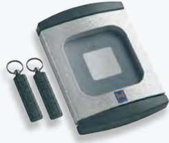
Transponder key switch in two versions TTR100/TTR1000 You simply hold the coded transponder key approx. 2 cm in front of the reader. Two keys are included, further keys are available on request. The comfortable TTR can recognise up to 100 keys and TTR 1000 up to 1000 keys.
